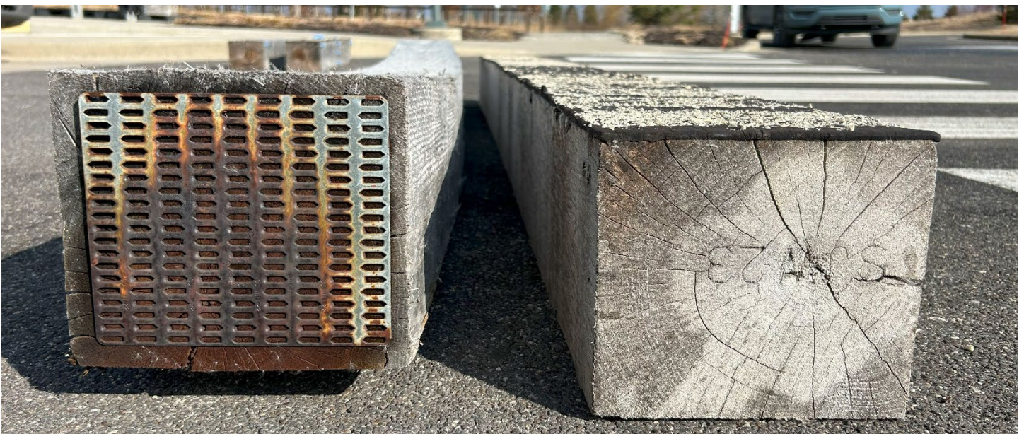
Uncoated Tie left vs. Tietan-coated Tie right
