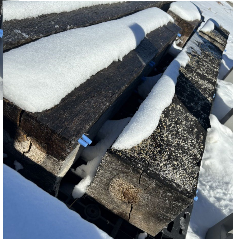
1/2 Length Ties: Uncoated vs. Tietan Coated
