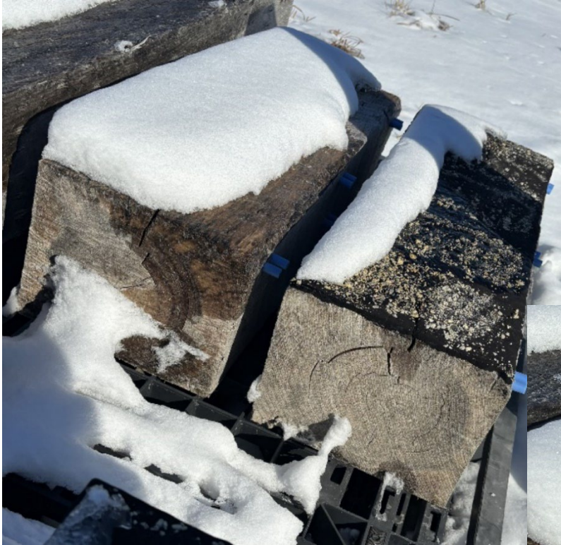
1/4 Length Ties: Uncoated vs. Tietan Coated
